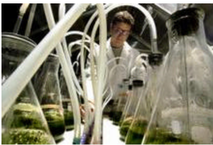
Blake Sherman, a research assistant for CSU spinoff Solix Biofuels, tends flasks of algae being tested for oil-conversion properties. Solix harvests the algae and crushes it into a type of vegetable oil that can be refined into biodiesel. CSU is shaping up as a supercluster school with several spinoffs that one day could become corporate giants.
